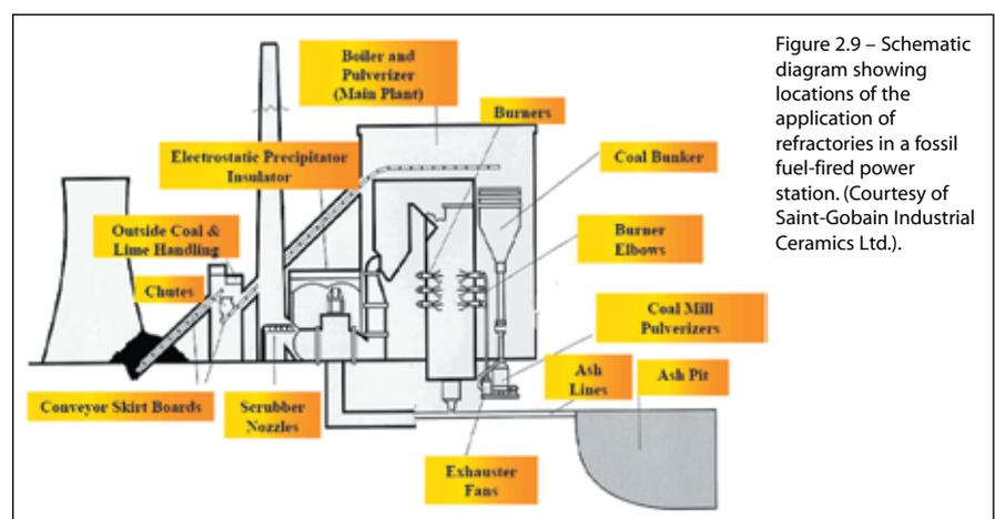
Figure 2.9 – Schematic diagram showing locations of the application of refractories in a fossil fuel-fired power station. (Courtesy of Saint-Gobain Industrial Ceramics Ltd.).
