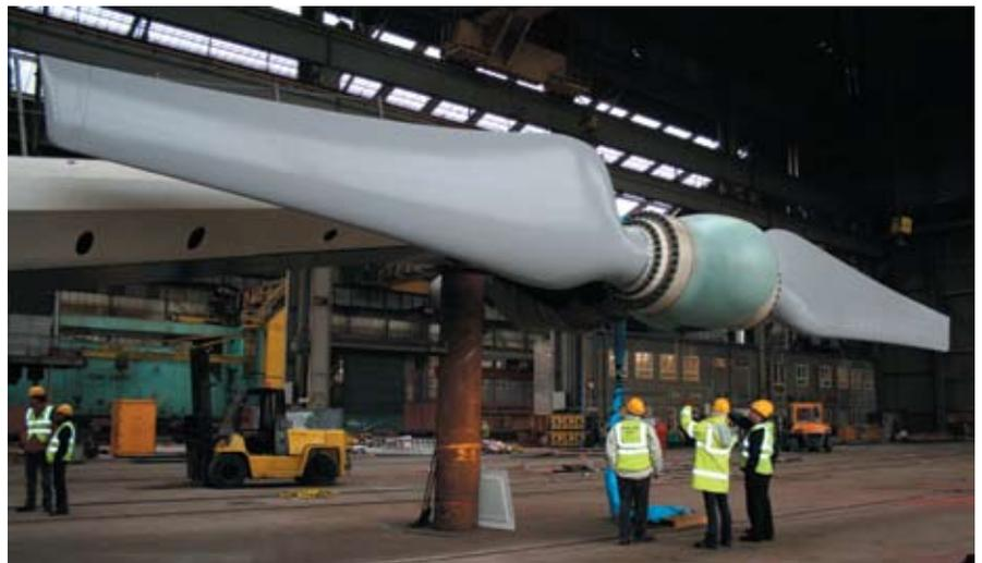
Figure 5.7 – Carbon fibre rotor blades for the 'SeaGen' tidal current turbine. (Courtesy of Marine Current Turbines Ltd: <http://www.marineturbines.com/>).
