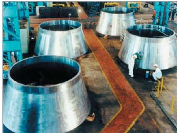
Figure 3.16 - Steam Generator transition cones. (Courtesy of Sheffield Forgemasters International Ltd.).
