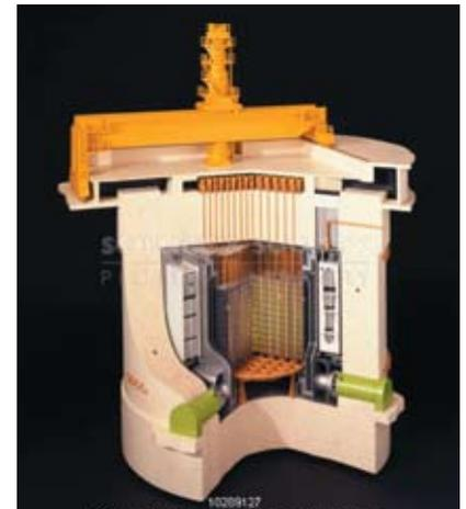
Figure 3.3 - Schematic of the Oldbury Magnox reactor, commissioned in 1968. (Courtesy of 'The Science & Society Picture Library': <http://www.scienceandsociety.co.uk/>)
