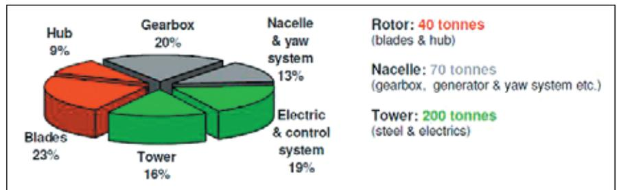
Figure 4.8 – Approximate weights and costs of wind turbine components. (Courtesy of BVG Associates Ltd.).
