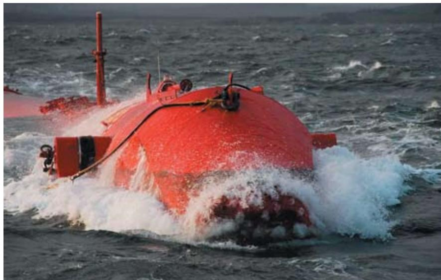
Figure 5.3 -The Pelamis Wave Energy Converter (WEC). (Courtesy of Pelamis Wave Power Ltd.: <http://www.pelamiswave.com/>).
