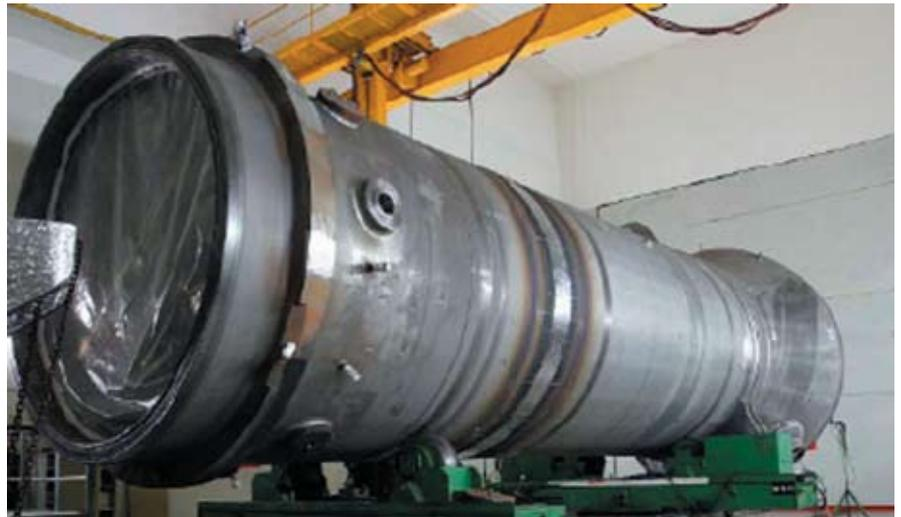
Figure 3.15 - Lower pressure boundary Steam Generator sub-assembly. (Courtesy of Areva NP).
