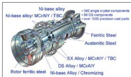
Figure 2.6 – Schematic of a gas turbine engine annotated with some of the materials of construction. (Courtesy of Alstom Power Ltd.).
