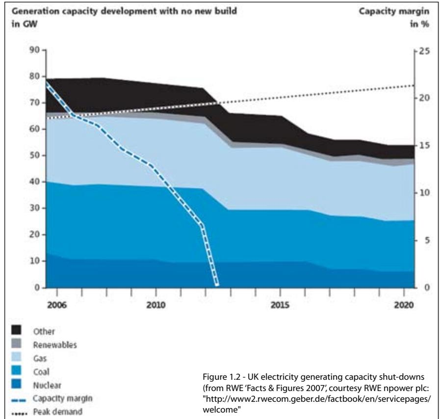
Figure 1.2 - UK electricity generating capacity shut-downs (from RWE 'Facts & Figures 2007', courtesy RWE npower plc: "http://www2.rwecom.geber.de/factbook/en/servicepages/welcome")
