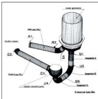
Figure 3.18 - Schematic diagram of Primary Loop (or Circuit) pipework for the Areva NP EPR. (Courtesy of Areva NP: <http://www.epr-reactor.co.uk/>).
