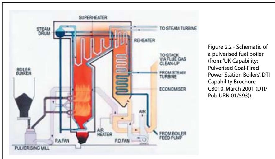
Figure 2.2 - Schematic of a pulverised fuel boiler (from: 'UK Capability: Pulverised Coal-Fired Power Station Boilers', DTI Capability Brochure CB010, March 2001 (DTI/Pub URN 01/593)).
