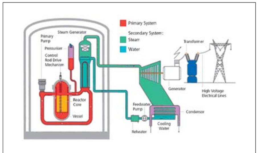
Figure 3.8 – Operational diagram of a typical PWR (from 'The UK Capability to Deliver a New Nuclear Build Programme', the NIA, March 2006. (Courtesy of the NIA: <http://www.niauk.org/>).
