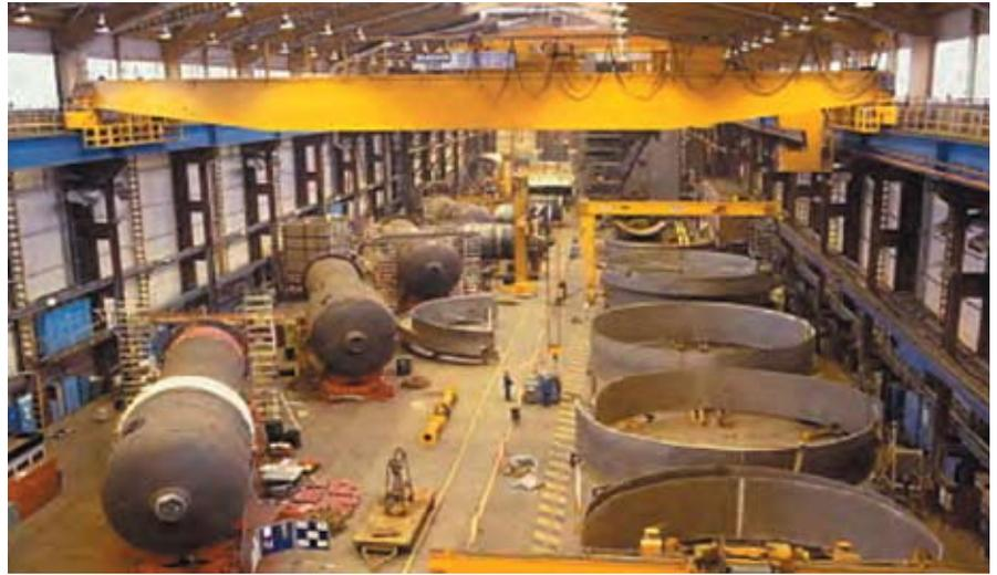
Figure 3.14 – Steam Generator fabrication at Mitsui (now Doosan) Babcock, Renfrew, for Sizewell B. (Courtesy of Doosan Babcock Energy Ltd.).
