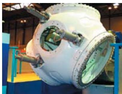
Figure 4.10 – A wind turbine nacelle bedplate casting. (Courtesy of 'WindSupply': <http://www.windsupply.co.uk/>).
