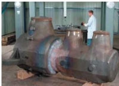
Figure 2.7 - Main stop valve body for a super-critical application, produced from two 10Cr-MoVWNbN, P911 castings, weld fabricated to make a 16,000kg valve body. (Courtesy Goodwin Steel Castings Ltd.).
