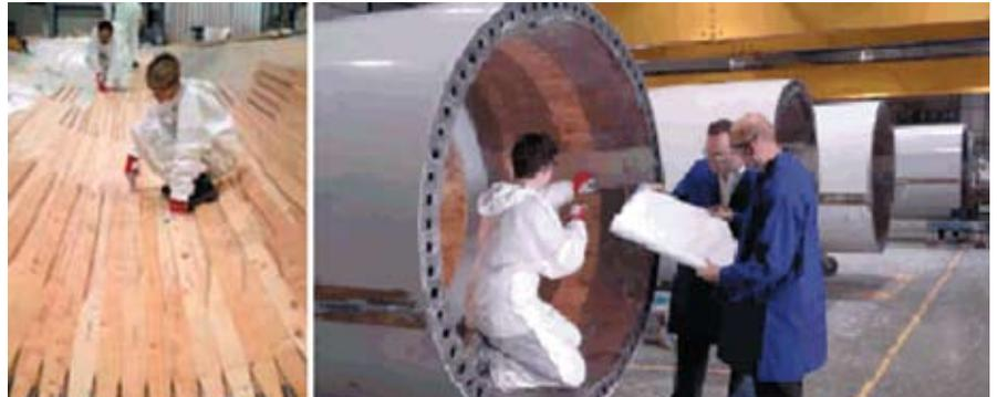
Figure 4.11 - Wind rotor blade fabrication at the Vestas Isle of Wight site. From: 'Environmental Statement 2006 – Company Site. Vestas Blades, Isle of Wight, England'. (Courtesy of Vestas: <http://www.vestas.com>).
